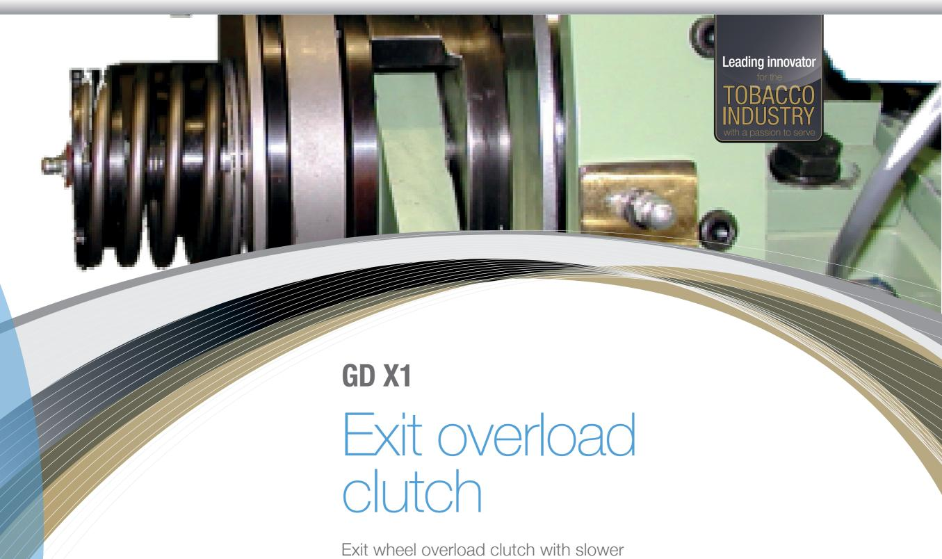
Exit wheel overload clutch with slower rotation when approaching the packet
